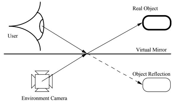
Fig. 3: Environment Mapping for Planar Objects
