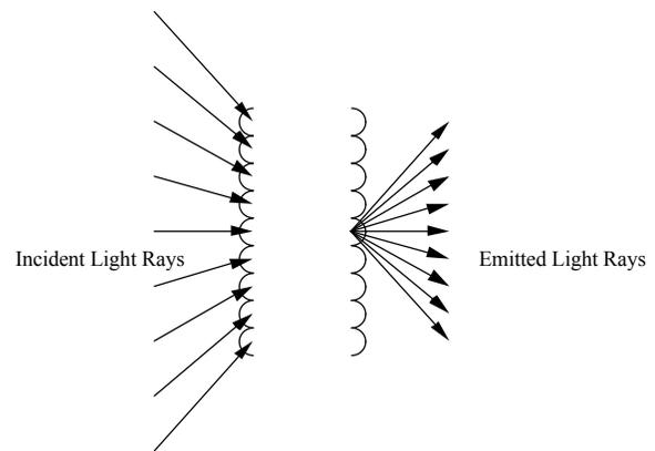
Fig. 6: Planar Two-Sided Planar Hyper-Display.
